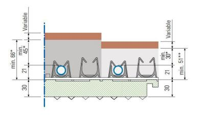
Guide-bar system for Ø 20pipes
