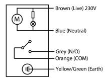
The auxiliary switch can be used as an interlock facility, thereby ensuring any auxiliary equipment is switched OFF when the valve is in the closed position. When the valve is in the fully open position the auxiliary equipment will be switched ON.\*
