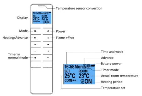
NOTE: This is thermostatic remote control. The remote should be in the same room as fireplace and placed on a flat surface. It must be placed away from the fire so the hot air will not blow on it and affect thermostatic reading.
