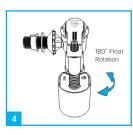
The valve has a float rotation system, allowing the float to be rotated 180°. This is really beneficial if space is an issue.
