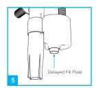
The valve comes with a delayed fill function which delays the filling of the cistern until 5 seconds (approx.) after the start of a flush.
