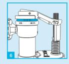
Refit top assembly complete with diaphragm and tun on water supply.
